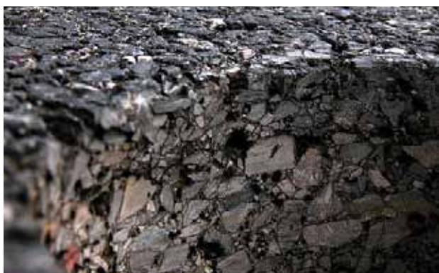
Photo 1: A typical core cross-section demonstrating the structural interlock of the RTM 10 – this offers increased rut resistance and shear strength due to a higher proportion of mid to large sized fraction.
